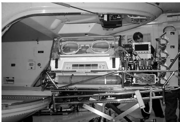
Figure 2 Top frame assembly locked into the starboard side of the aircraft.
