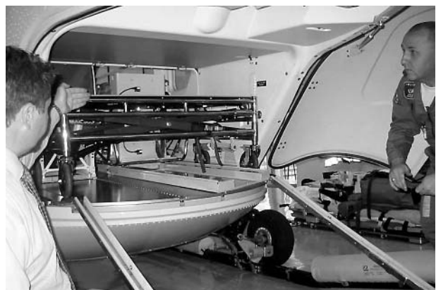
Figure 3 Trolley base loaded in the aft of the helicopter.
